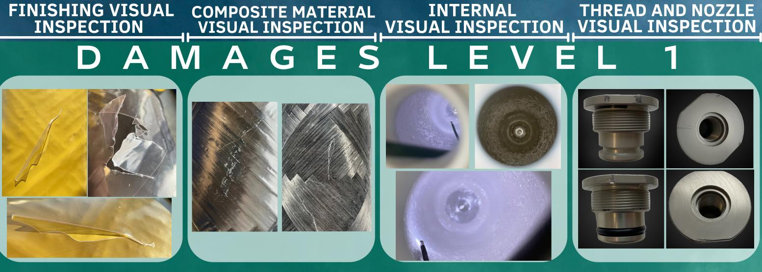
DAMAGES LEVEL 1: This kind of damages on the cylinders are classed as Level 1 damageand are acceptable, hence no repair is required. Such damage has no adverse effects on the safety of the cylinder and its continued use.
