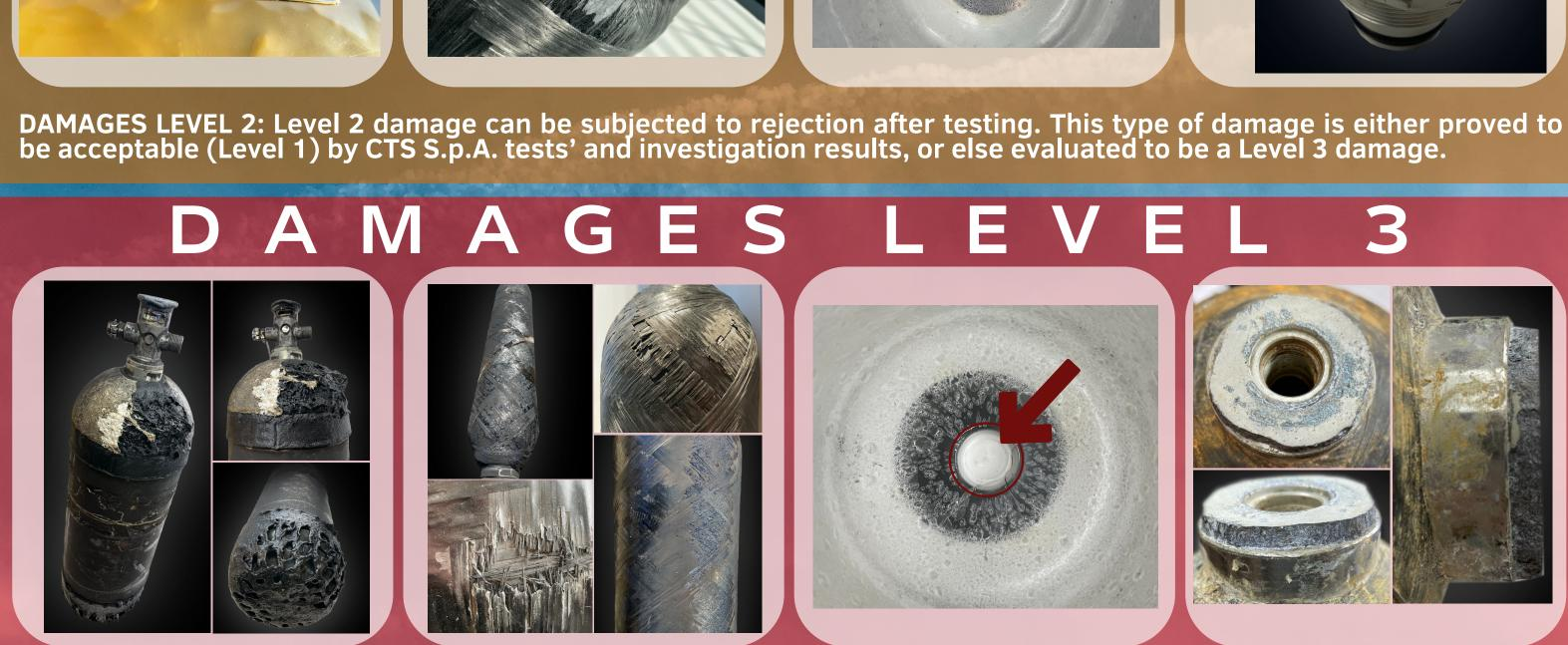
DAMAGES LEVEL 3: Level 3 damage is sufficiently severe that the cylinder cannot be repaired: it shall be rejected and subsequently made unserviceable.
