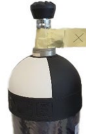
Fig.7: Cylinder with open valve and anti-tampering tape
