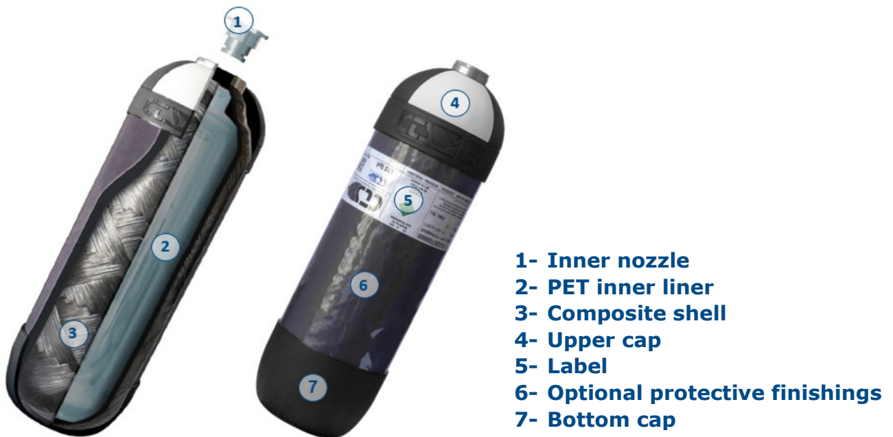
Figure 1. CTS cylinder composition diagram
