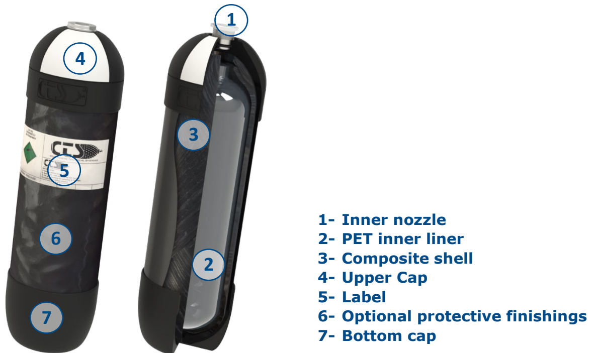
Figure 1. CTS cylinder composition diagram
