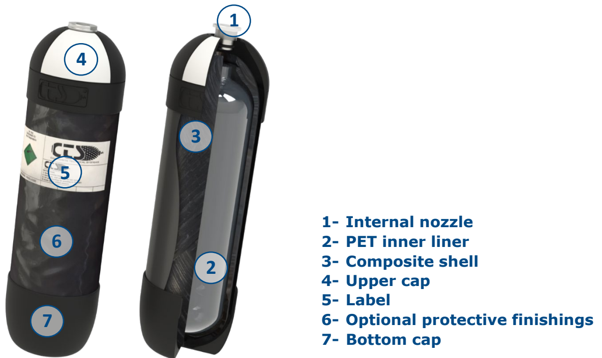
Figure 1. CTS cylinder composition diagram
