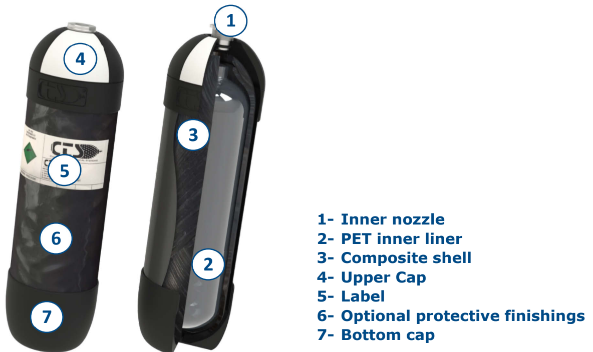
Figure 1. CTS cylinder composition diagram
