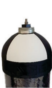
Fig.4: Cylinder with valve and internal pressure of 29 psi
