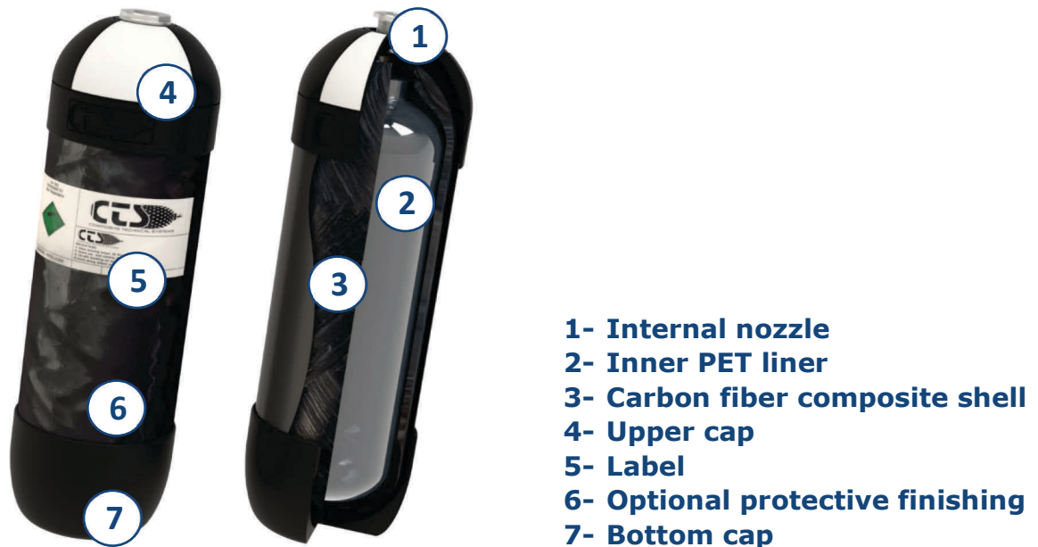
Figure 1. CTS cylinder composition diagram
