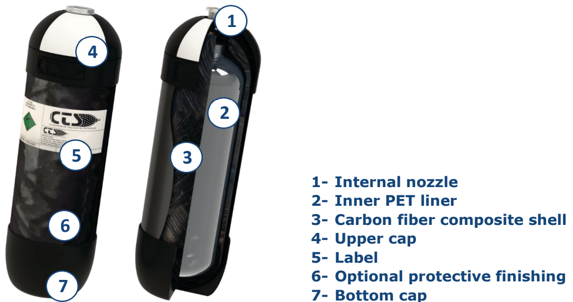
Figure 1. CTS cylinder composition diagram
