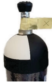
Fig.7: Cylinder with open valve and anti-tampering tape
