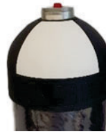
Fig.6: Cylinder with cap and without internal pressure
