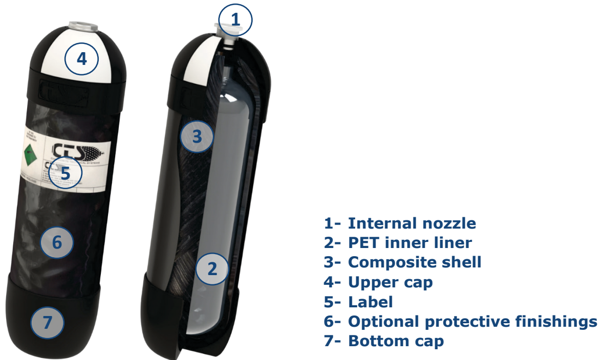
Figure 1. CTS cylinder composition diagram
