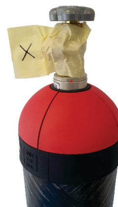
Fig.7: Cylinder with open valve and anti-tampering tape
