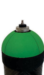
Fig.4: Cylinder without valve and internal pressure of 2 bar
